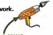
**POWER RATING** — amount of energy an appliance transfers per second when working at its recommended maximum power.
